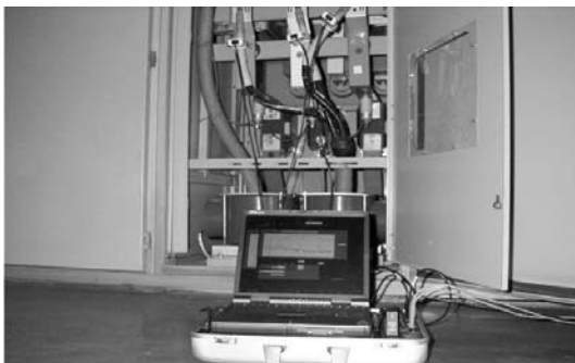
Fig. 7 Current analysis of running motor
